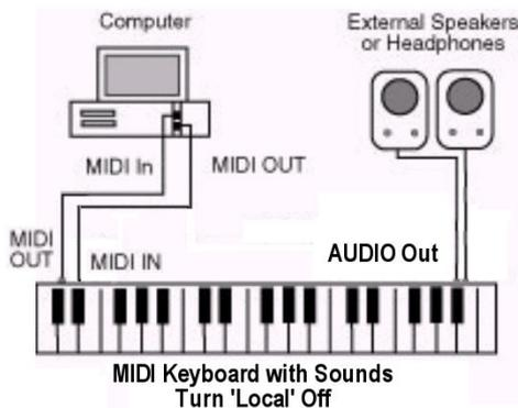
c.i. Using a MIDI keyboard (synthesiser or sampler) instead of a MIDI module, as (b) above.
