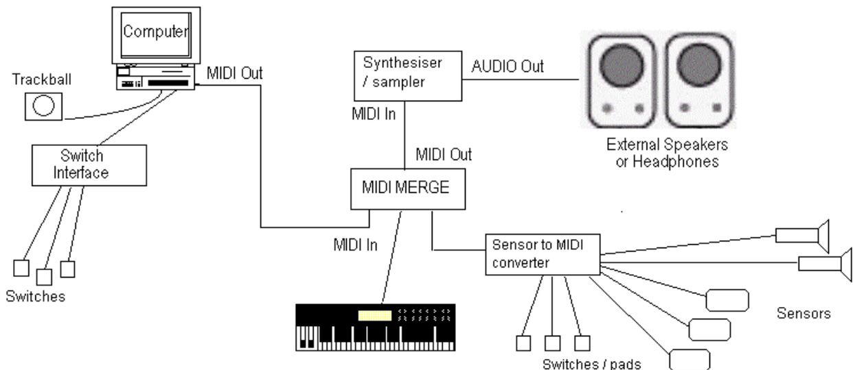
(e) Using E-Scape as the master instrument with MIDI module and multiple controllers
